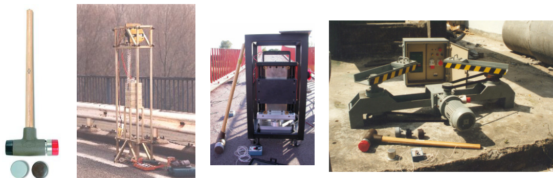
Fig. 1. a) Impulse hammer; b) Impulse excitation device for bridges (K.U.Leuven); c) Electrodynamic shaker over three load cells; d) Eccentric mass vibrator.
