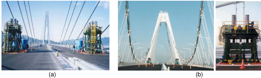
Fig. 10. Forced vibration tests of (a) Tatara cable-stayed bridge ( http://www.hsba.go.jp ) and (b) Yeongjong suspension bridge ( http://www.yeongjongbridge.com )
