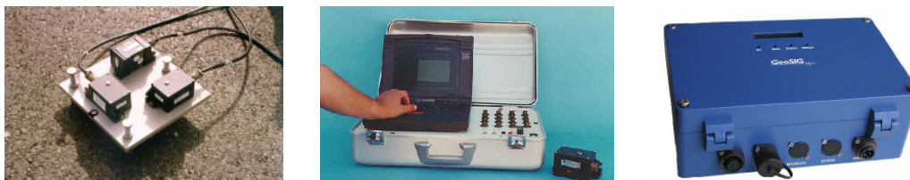
Fig. 11. (a) Force balance accelerometers; (b) Multi-channel data acquisition and processing system for ambient vibration tests; (c) Strong motion tri-axial seismograph
